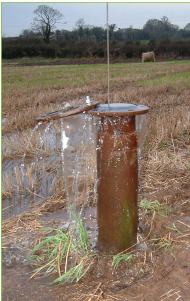
PICTURE ABOVE: Artesian borehole being geophysically logged
